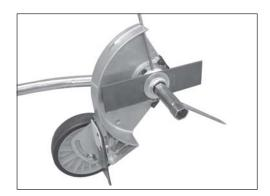
3. Rotate blade until holes in inner blade adapter (B) and gear box align. Insert locking tool to lock PTO shaft (C).
